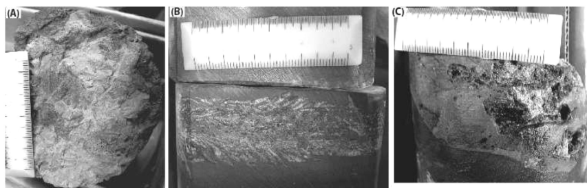
Figure 10. A) Bedding plane view of bedded nahcolite (125.58 m depth in Figure 4). B) Small nahcolite vugs (113.45 m depth in figure 4). C) Large nahcolite vugs (122.83 m depth in figure 4). Note that scale is 5 cm long in all photos.
