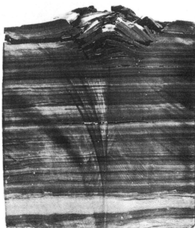
Figure 2. Thermomechanical fragmentation in a 1-ft cubic block heated with one face exposed to steam flowing at 520 °F. The block was confined on all faces except the one that underwent fragmentation. Reprinted by permission from reference (4). Copyright 1977 Society of Petroleum Engineers.
